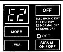
When E1, E2 (shown) or E3 appears in the display, the dryer is operating in the electronic drying mode.
